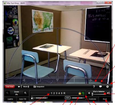
**Speed gauge** – an indicator of the VGo's speed where 1 is slowest and 5 is fastest
