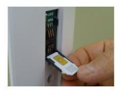
3) Position the SIM card with the metal contacts facing up and the notched corner on the left. Slide the SIM card into the back of the cover, and fold the cover back up into the stalk.
