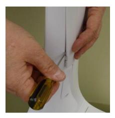
1) Using a small flathead screwdriver or knife, starting at the bottom, gently pry off the plastic screw cover strip on the left inside stalk of the VGo.
